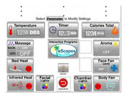
**Cabinet Temperature**: The user can change the settings for the cabinet temperature at any time during the session by simply pressing the Temperature box which will bring you to the change temperature screen as shown:
